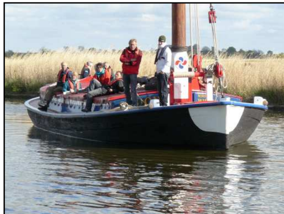
Albion coasting in – note the white bow a feature of the wherry. Seeing the white in the distance in a narrow waterway tells you it's approaching.
